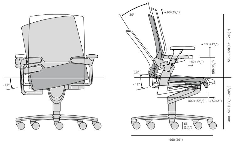
Due to innovative, synchro-supporting 3D kinematics (Trimension®), the sideways inclination of the seat and backrest is integrated into a perfect and synchronous movement concept.
